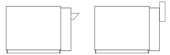
When the chimney and flue cap are provided by others, install in accordance with the instructions for the chimney and flue cap and to the requirements of the authorities having jurisdiction. The chimney shall a Category II Type "BH" vent and be suitable for outdoor installation. Support the chimney independent of the unit.
