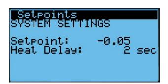
Controller vent pressure setpoint. The default setting is -0.05. This setpoint should not need to be altered.
