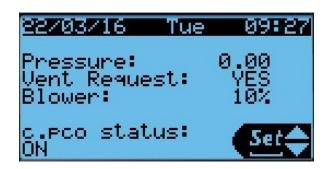
The main display mask shows the present date and time, the actual measured pressure, the request to operate from the heating device combustion fan, and the power vent fan motor current operating speed.
