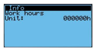
Displays the operational time of the controller and program. This is not the total powered time of the control.
