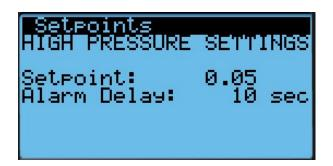
The high (over) pressure setpoint and alarm delay. Setting is set to just slightly positive pressure with a 10 second delay before locking out the system.
