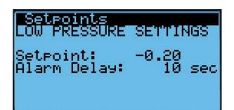
The low pressure setting and alarm delay. If the control operates below this setpoint for more than 10 seconds the control will lock out the system and go into alarm condition.
