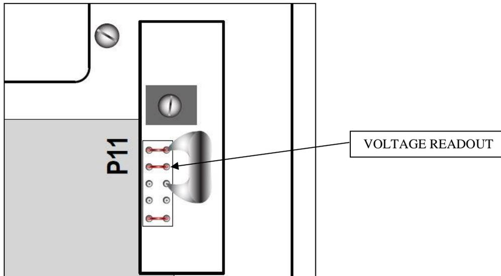
This adjustment ensures that the internal temperature control reset curve starts just as the VFD begins to ramp up. The internal reset signal will be at maximum when the AFB voltage has increased by 6 VDC greater than the minimum volume voltage. If the minimum input voltage is greater than 4 VDC the amount of the internal temperature reset is reduced.
