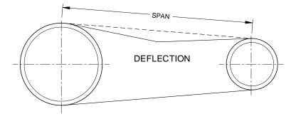
A CAUTION: Excessive belt tension is the most frequent cause of belt wear, bearing wear and noise.
