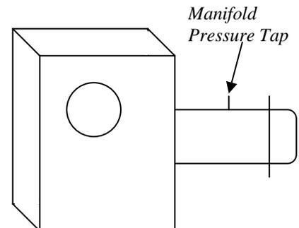
On some indoor units the vent orifice fitting on the RV appliance regulator is to be vented to atmosphere. The field installed vent line should be sized adequately especially on longer runs. If there is more than one regulator connected to a common run that includes the main regulator, and the line is not adequately sized, an erratic inlet pressure will result and cause improper combustion and also burner pulsating problems.
