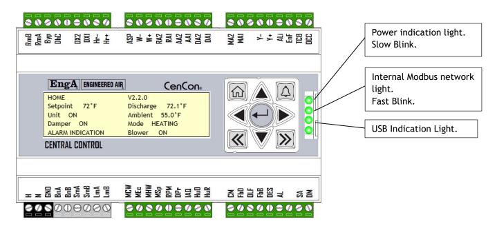
The Engineered Air CenCon controller is the primary operational component for the majority of custom manufactured Engineered Air HVAC equipment. Various expansion modules (-XM) may be added to extend the operational capabilities to gas fired heating, cooling, humidification, and energy recovery systems.
