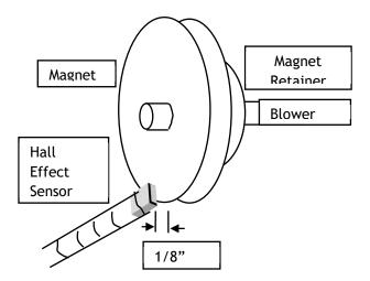
With a digital AC voltmeter, measure the AC volts present on terminals "YS to GS". When the combustion blower is running there should be 4 to 6 Vac present. If the AC voltage is not present, confirm the tachometer sensor is located near the circumference of the magnet, with a 1/16 to 1/8" (2-3mm). Ensure speed sensor wire is routed at least 8" (200mm) away from any power wiring.
