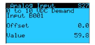
Analog inputs can be calibrated with offset values when a sensor error is found.
