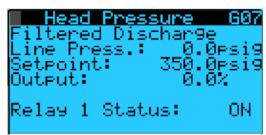
This mask is visible if head pressure control is enabled. Filtered discharge pressure, pressure set point, analog output capacity, and relay status are shown.
