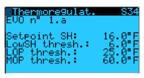
Superheat and other adjustible EVD setpoints are available. Superheat control is critical to the operating life of a digital compressor. Only qualified personnel should adjust these settings.
