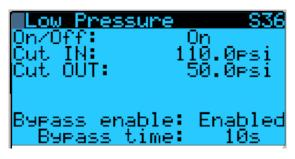
Low pressure control cut in and cut out set points are adjustable. The bypass timer mitigates nuisance trips cause by normal pressure fluctuations with digital systems. Low pressure allows three trips in a one hour period before requiring a manual reset.
