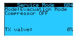
While using Evacuation Mode the EEV opens to 100% (may delay depending on previous compressor state), compressor is locked out.
