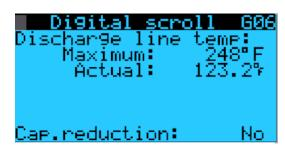
The discharge line temperature is displayed. If capacity reduction is shown to be on (yes), the controller will reduce capacity to prevent compressor overheating.
