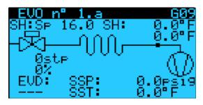
Operation status of the EVD controller is displayed. Superheat, suction pressure/temperature and valve information is provided. When a Twin EVD is used, information for both valves is displayed.
