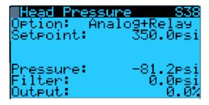
There are several head pressure control options available. The specific option can only be changed from the manufacturing menu with individual settings able to be adjusted from the service menu. There are 6 different head pressure options which have different standard settings.
