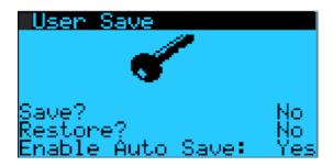
Allows user settings to be saved. When the pCO controller is powered up it will use variables from the last saved user input.
