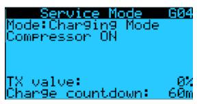
While using Charging Mode, the EEV is enabled, compressor operates at 100%, and low pressure cut out set to 5 PSI. Charging mode will automatically exit when countdown has ran out (default 60 minutes).
