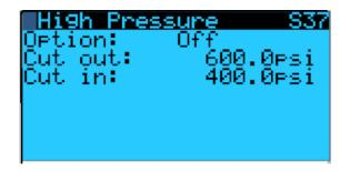
High pressure control cut in and cut out set points are adjustible. This pressure control can be set as manual reset, auto reset, or three auto trips over a selecteble time.
