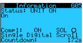
The main display indicates requested demand, and Digital output capacity. If a second compressor is enabled, the display will show when it is running.
