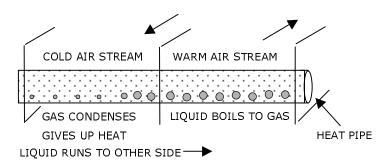
The heat pipe is a device that transfers heat through a fluid media enclosed in a pipe without any mechanical work being performed (such as the use of a compressor or burning fuel). When one part of the heat pipe is located in a warmer ENGINEERED AIR®
