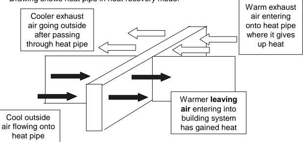
Drawing shows heat pipe in heat recovery mode.
