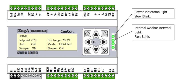
The Engineered Air CenCon controller is the primary operational component for the majority of custom manufactured Engineered Air HVAC equipment. Expansion modules (-XM) may be added to extend the operational capabilities to gas fired heating, cooling, humidification and energy recovery systems.
